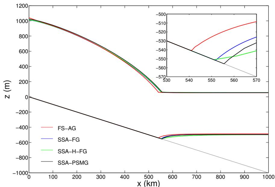
FIGURE 3.8 – Initial steady state geometry ( $C_F = 0.4$ ) for all models. The inset emphasizes the differences in GL position. **SSA-H-FG** lower surface has a quite different shape with respect to the three other models due to its coarser resolution (10 km).
