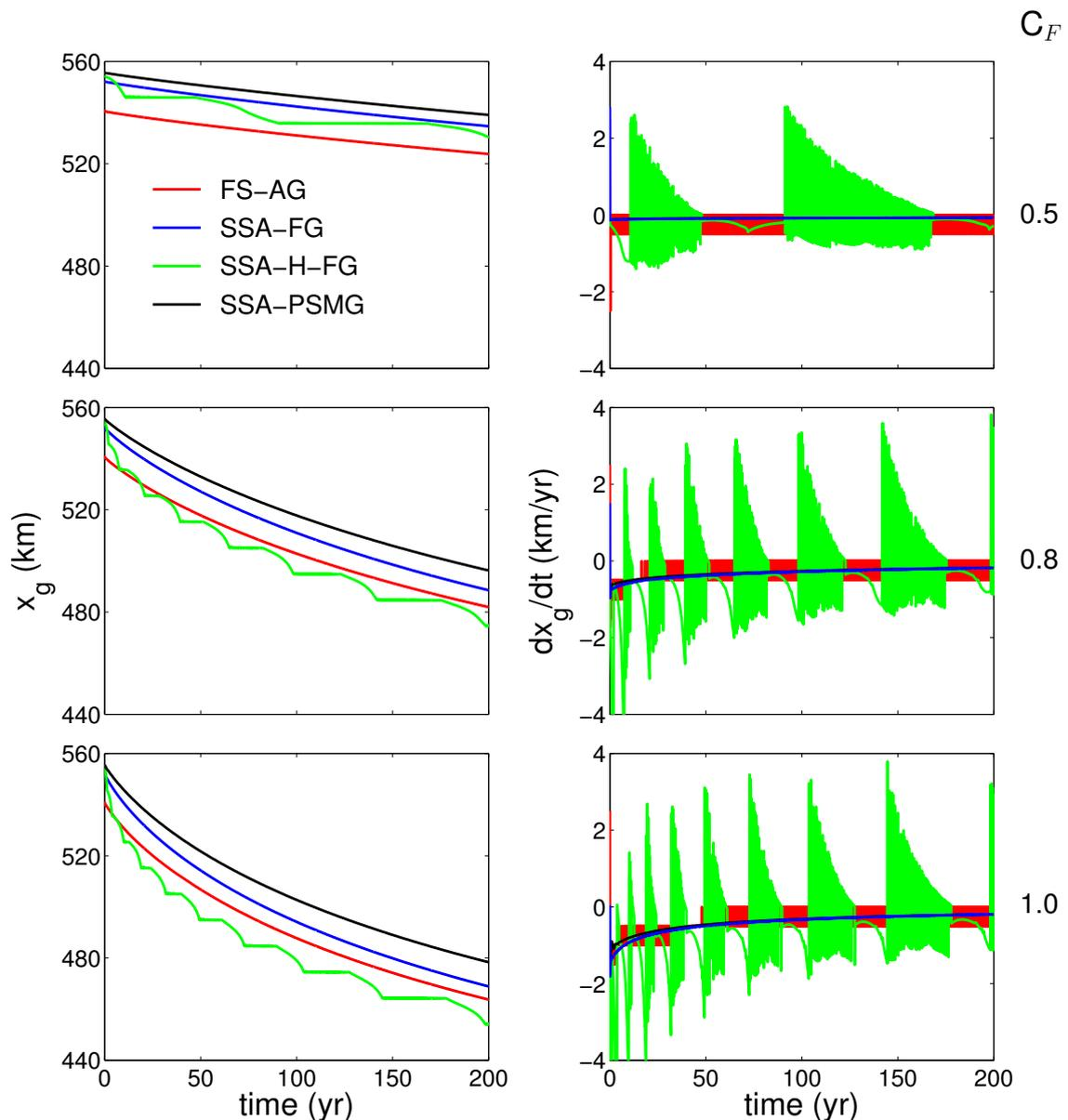
FIGURE 3.9 – Grounding line position  $x_g$  (left) and migration rate  $dx_g/dt$  (right) as a function of time for the four models and for the three buttressing values ( $C_F = 0.5$  on the first line,  $C_F = 0.8$  on the second line and  $C_F = 1$  on the third line).
