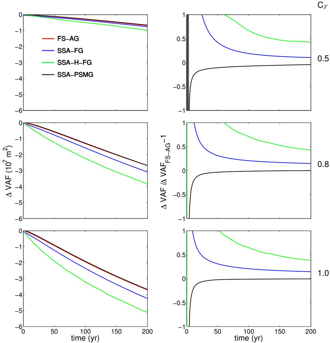
FIGURE 3.13 – Temporal evolution of the variation of Volume above Flotation ( $\Delta VAF$ ) for each model (left) and, expressed relative to **FS-AG** ( $\Delta VAF_{\text{FS-AG}}$ ) for the three remaining models (right), for the three butressing values (lines).
