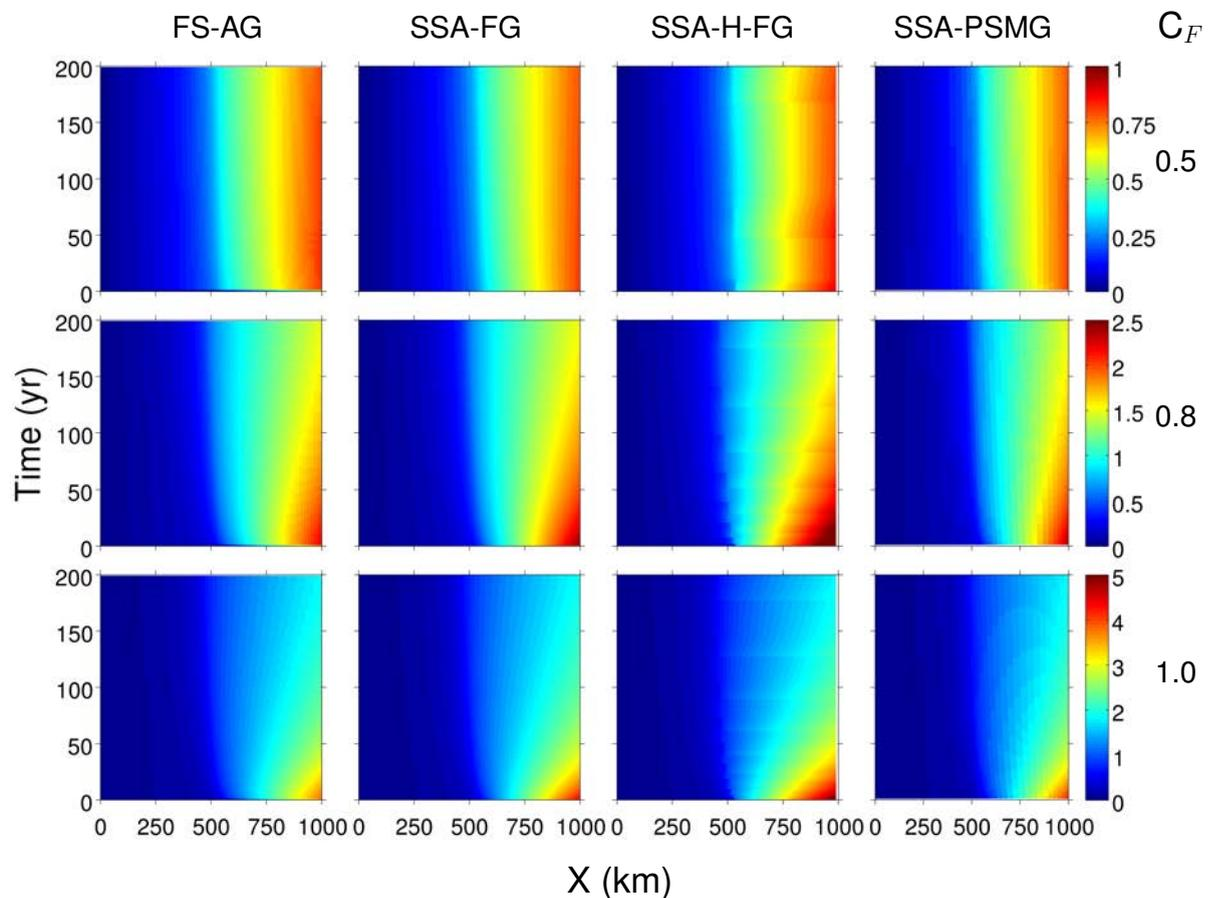
FIGURE 3.11 – Surface horizontal velocity ( $\text{m yr}^{-1}$ ) as a function of time and horizontal distance ( $x = 0$  corresponds to the ice divide and  $x_f = 1000$  km is the calving front) for the three buttressing values (lines) and for the four models (columns).
