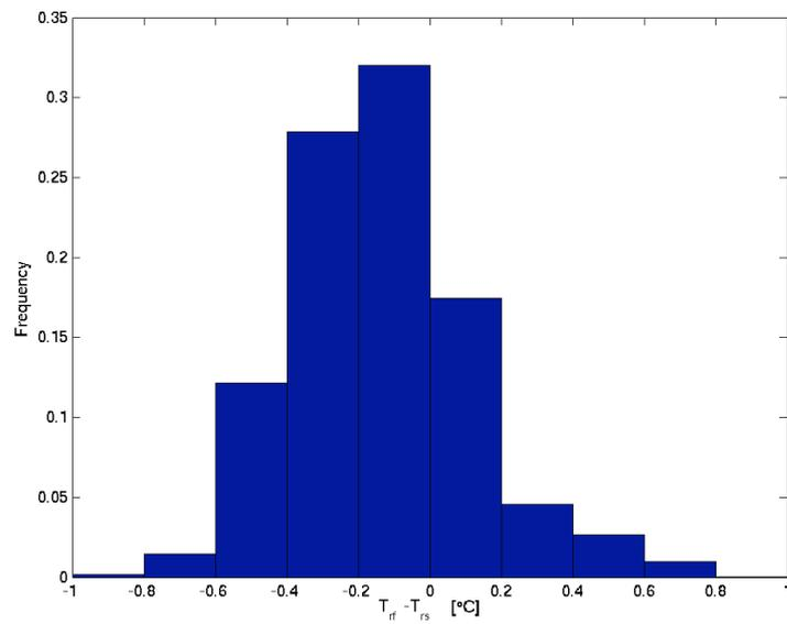
**Figure 2.2** Distribution of the temperature differences between the Rosemount 102 ( $T_{rs}$ ) and the reverse flow temperature ( $T_{rf}$ ) probes for all ice clouds defined in Table 2.1.
