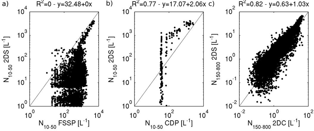
**Figure 2.3** FSSP concentration as function of 2DS concentration (a), CDP concentration as function of 2DS concentration (b) (10-50  $\mu\text{m}$ ) for ice clouds defined in the Table 2.1 with  $T_a < -15$   $^{\circ}\text{C}$ . 2DC concentration as function of 2DS concentration (c) (150-800  $\mu\text{m}$ ) for ice clouds defined in the Table 2.1.
