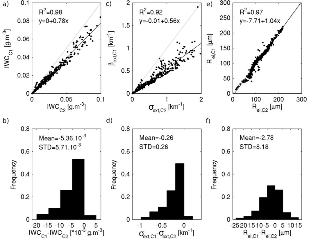
**Figure 2.4** Comparison of  $IWC$  (a,b),  $\sigma_{ext}$  (c,d) and  $R_{ei}$  (e,f) from combinations (1) 2DS for  $N_{10 < D < 150 \mu m}$ , 2DC for  $N_{150 < D < 800 \mu m}$ , 2DP for  $N_{D > 800 \mu m}$  and (2) 2DS for  $N_{10 < D < 800 \mu m}$ , 2DP for  $N_{D > 800 \mu m}$  for ice clouds defined in the Table 2.1.
