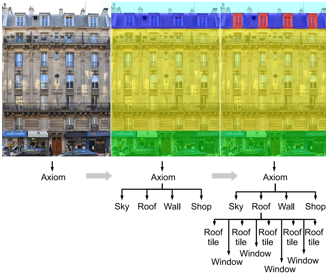
Figure 8.1: Top-down construction of a derivation tree. Top: the input image with the overlaid symbols. Bottom: the derivation tree under construction.
