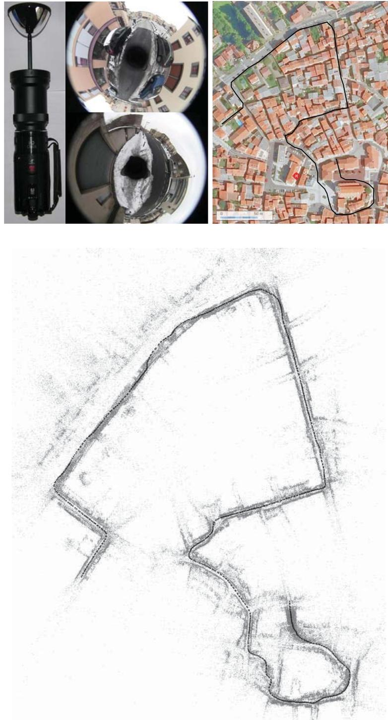
**Figure 7.14:** Overview of incremental SfM. At the top, we see from left to right: the catadioptric camera, two sequence images and aerial view of trajectory. At the bottom, we see the final reconstructed SfM points and camera poses.
