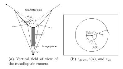
Figure 3.4: Vertical field of view of catadioptric camera.
