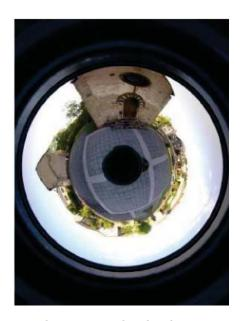
**Figure 3.2:** A catadioptric camera and an image taken by this camera.
