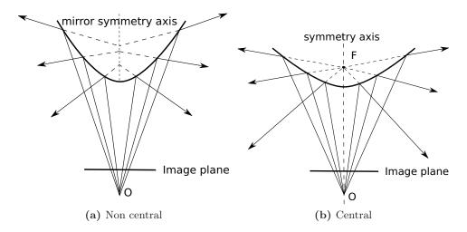
Figure 3.3: Non central and central catadioptric camera models
