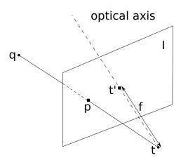
**Figure 3.1:** Perspective camera model.  $\mathbf{q}$  is a 3d point,  $\mathbf{p}$  is the projection of  $\mathbf{q}$  on image plane, f is the focal length,  $\mathbf{t}$  is the center and  $\mathbf{t}'$  is the principal point.
