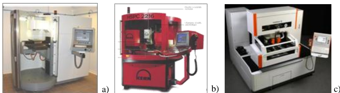
Figure 56. Equipment used in the investigation related to the machining of die cavities, a) DML 40 SI laser micro-manufacturing; b) HSPC 2216 high speed micro-milling and c) Charmilles Robofil 2050TW micro-Wire Electrical Discharge equipment
