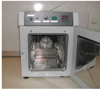
Figure 69. Thermal debinding oven used in our analyses
