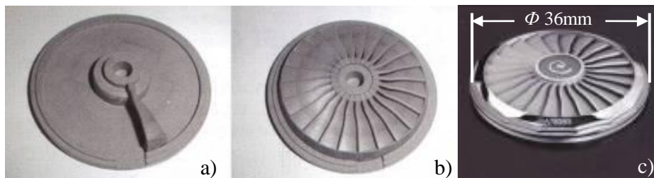
Figure 25. Production process for the aerospace turbine engine themed watch case realized by Alliance ® (courtesy of EPMA), a) injected individual blade and support; b) 24 injected blades and injected support and c) sintered component
