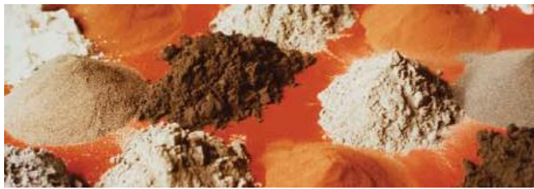
Figure 11. Examples of the metal powders used for MIM process [9]
