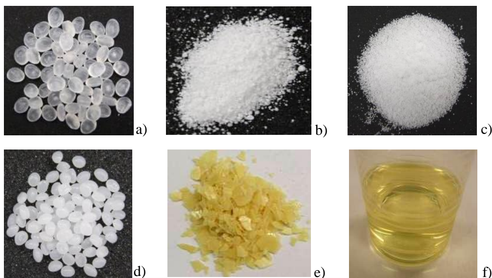
Figure 32. Examples of binder used in the feedstock, a) PP_A, granular of 3~4 mm; b) LDPE_G, powder of 1 mm; c) SA, powder of 0.2~0.3 mm ; d) LDPE_A, granular of 2.5~3.5 mm; e) CW_A, lamellar; f) OA, liquid
