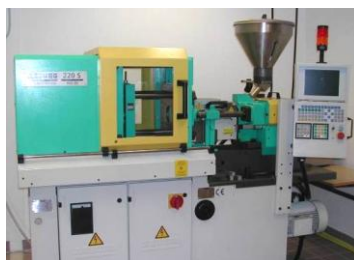
Figure 53. Hydraulic Arburg 220-S injection equipment for the conventional injection molding
