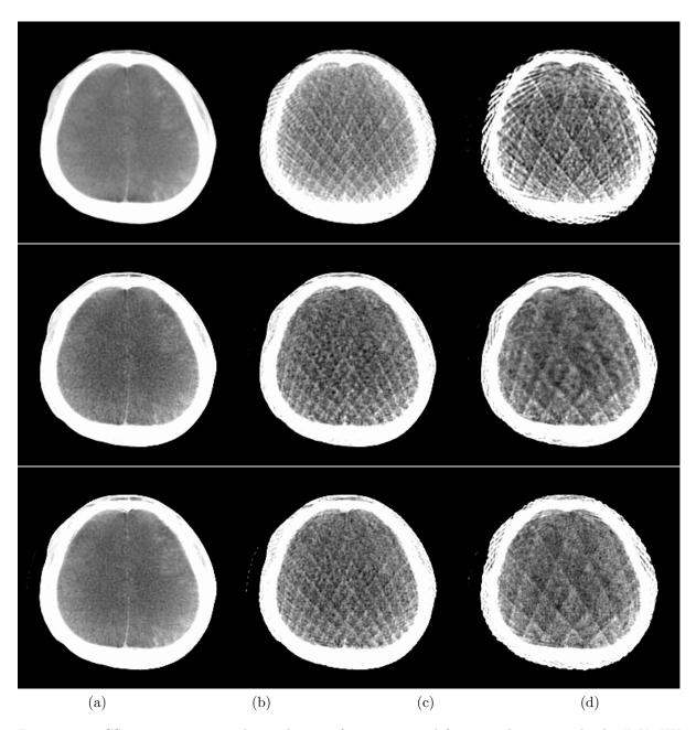
Figure 4.20: CS reconstruction and sampling artifacts originated from an object outside the FoV. HU range: 950 to 1200. First row: iFDK+ reconstruction. Second row: CS – sbs reconstruction. Third row: CS – tv reconstruction. Sampling rate: (a) 600 views. (b) 150 views. (c) 75 views.
