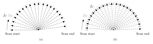
Figure 5.3: DSRA acquisition protocol design. The mask angular sampling pattern is plotted with dashed gray arrows, while the contrast angular sampling pattern is plotted with dashed black arrows. (a) Homogeneous acquisition: contrast and mask scans sample the same set of equiangularly spaced positions. (b) Heterogeneous acquisition with  $\delta = 0.5\Delta\phi$ : contrast and mask scans sample two sets of equiangularly spaced interleaved positions.
