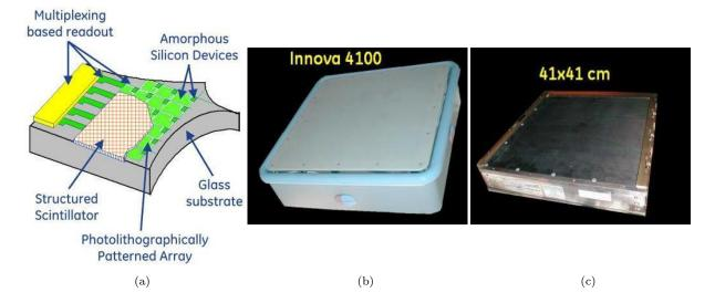
Figure 3.3: (a) Schematic representation of the layers that compound the sensor used in flat-panel detectors. The detector is based on a crystalline CsI scintillator and an a-Si diode. Active readout matrix includes readout electronics based on a small thin-film transistor. (b) Photograph of the flat panel detector of Innova 4100 with its packaging. (c) Photograph of the flat panel detector of Innova 4100.
