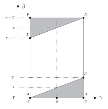
Figure 2.18: Short scan. Sinogram measurement plotted in the  $(\beta, \gamma)$  domain.
