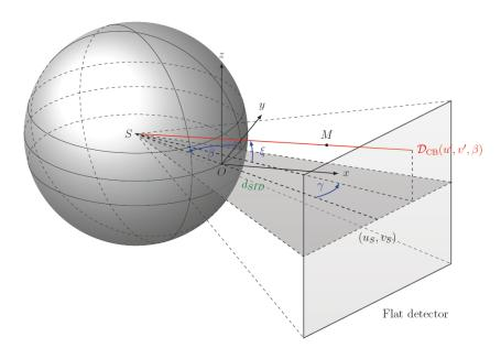
Figure 3.5: Coordinate systems in cone-beam geometry.
