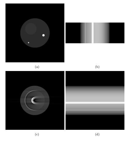
Figure 5.2: Toy example. (a) 2D numerical phantom. (b) Simulation of the sinogram acquired in parallel geometry with 150 integral lines while the phantom is rotating at the same speed as the system gantry. (c) FBP reconstruction. (d) Motion-compensated reconstruction.
