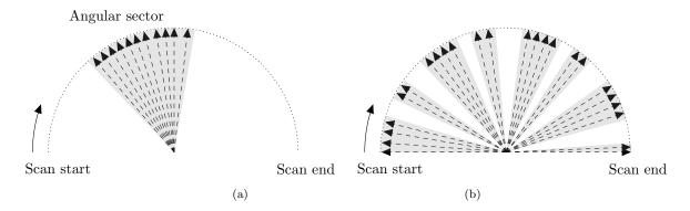
Figure 2.8: (a) Limited angle sampling subset. (b) Nonuniform subsampling subset.
