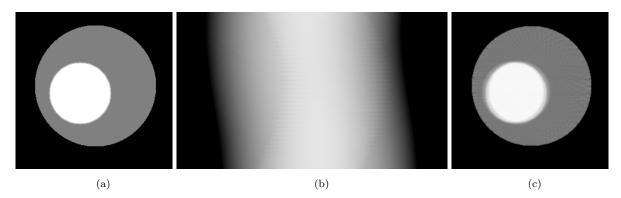
Figure 2.10: Motion artifacts with low contrast structures (a) Imaged object with background of value 1000 and moving structures of contrast 100 - display range: 900 to 1110. Simulation of a parallel-beam sinogram with 300 equiangularly spaced integral lines over 180°. Uniform periodic displacement of the moving structure: (b) sinogram; (c) static FBP reconstruction.
