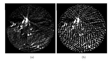
Figure 5.4: Impact of the acquisition protocol on the subtracted volume (N=75 views). (a) FDK reconstruction for the homogeneous protocol: the redundant background structures and the associated streaks are removed. (b) FDK reconstruction for a heterogeneous protocol ( $\delta=0.5\Delta\phi$ ): streaks associated to the background structures cannot be removed. Vessel streaks remain with both protocols.
