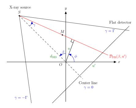
Figure 3.7: Coordinate systems in fan-beam geometry with a flat detector.
