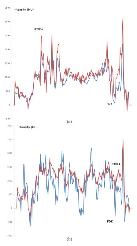
Figure 4.4: Comparison of FDK and iFDK+ with regard to the sampling rate. Intensity profile curves drawn through the axial slice presented in Fig. 4.3 for (a) the full scan (about 150 views) (b) a subsampling factor equal to 8. Reconstruction using FDK is plotted in blue, while reconstruction using iFDK+ is plotted in red.
