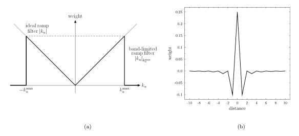
Figure 2.4: Band-limited ramp filter: (a) frequency response, (b) impulse response.
