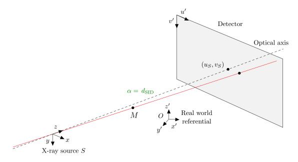
Figure 3.6: Cone-beam geometry. Ideal acquisition: x, z, x', y' and u' belong to the same plane and z', v' and y are aligned.
