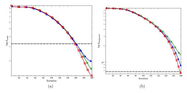
Figure 5.14: Convergence curves (RMSD values) for the numerical phantom with pulsatile motion: prior image (black dashed line), CS-sbs (green circles), CS-piccs (blue triangles) and CS-sbs+t (red squares). (a) RoI with dynamic injected vessels over static background for phase 1; (b) RoI with static structures.
