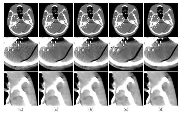
Figure 4.9: Reconstruction results with positivity and with regularization strategies. First row: reconstructed image. Second row: zoomed detail with HU range from 850 to 1230. Third row: zoomed detail with HU range from 600 to 1200. Reconstruction result of: (a) experiment n°1. (b) experiment n°2. (c) experiment n°3. (d) experiment n°4. (e) experiment n°5.
