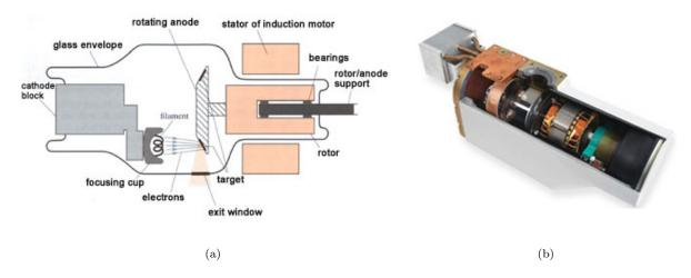
Figure 2.12: (a) Schematic representation of the elements of an X-ray tube [1]. (b) Photograph of an X-ray tube (GE Healthcare, Chalfont St. Giles, UK).
