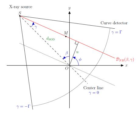
Figure 2.17: Coordinate systems in fan-beam geometry with a circular detector.
