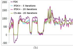
Figure 4.18: Intensity profile curves for comparison of positivity constraint and SBS in the non-subtracted case: (a) through the axial slices shown in Fig. 4.16, (b) through the sagittal slices shown in Fig. 4.17.
