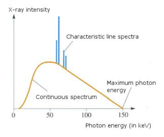
Figure 2.13: Spectrum emitted by the X-ray tube for visualization of biological tissues with an operating voltage of 150 kV and a tungsten target. The continuous spectrum of Bremsstrahlung emission is plotted in orange, while radiations characteristic of the target material are superimposed in blue.
