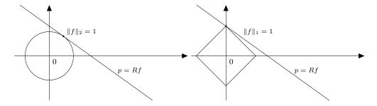
Figure 4.1: Geometric interpretation of the  $\ell_1$  and  $\ell_2$  norms. (a)  $\ell_1$  ball: the anisotropy of the  $\ell_1$  ball favors sparse solution. (b)  $\ell_2$  ball: minimizing the  $\ell_2$  norm generally does not allow for recovery of sparse solutions.
