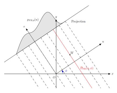
Figure 2.1: Coordinate systems in parallel-beam geometry.
