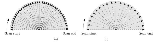
Figure 2.5: Angular sampling patterns. (a) Full sampling. (b) Uniform subsampling.
