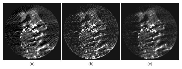
Figure 4.14: Visual comparison between FDK, positivity constraint and SBS in the subtracted case. HU range: 550 to 1050. (a) FDK reconstruction. (b) iFDK+ reconstruction. (c) CS – sbs reconstruction.
