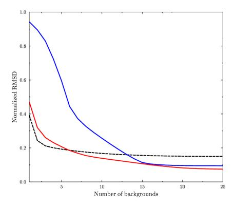
Figure 5.23: Convergence curves (RMSD values) for the numerical phantom. Reconstructions: CS-piccs (black dashed line), CS-sbs+t (blue line), CS-wm+tv (red line).
