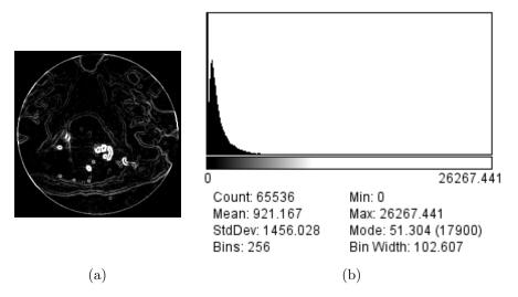
Figure 4.6: Sparsity in the gradient domain. (a) Gradient image of a C-arm CT slice. (b) Corresponding intensity histogram.
