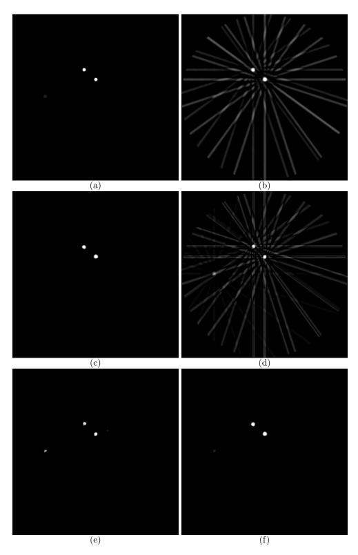
Figure 4.2: Illustration of OMP principle. (a) Sparse phantom. (b) FDK reconstruction from 10 views. (c) Detected components after thresholding. (d) FDK reconstruction of the residual. (e) Detected components after thresholding. (f) Final reconstruction: sum of (c) and (e).
