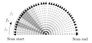
Figure 5.1: Dynamic data acquisition model: the temporal variations encountered during the acquisition within a 2-phase object are modelled as a succession of phase  $f_0$  (in light gray) and phase  $f_1$  (in dark gray).
