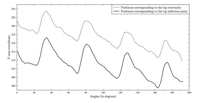
Figure 3.26: Evaluation of the dynamic of the motion in a scan. Manual identification of the temporal signal that is associated to the motion of the catheter.
