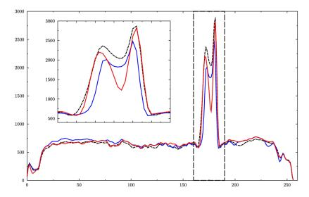
Figure 5.16: Reconstruction results for the pulsatile motion case. Intensity profile curves drawn through the axial slices shown in Fig. 5.15: static reconstruction (black dashed line), CS-sbs+t for phase 1 (blue plain line) and phase 2 (red plain line).
