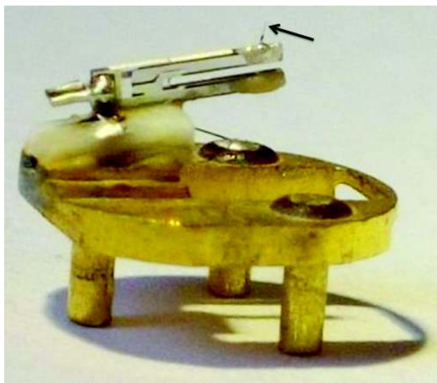
FIG. 1. (Color online) Optical image of the tuning fork probe mounted on a modified VT-AFM Omicron holder. The black arrow indicates the location of the etched Pt/Ir tip.
