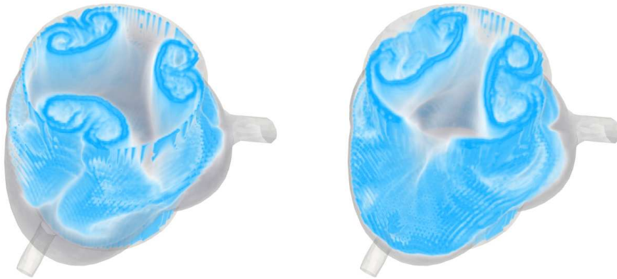
Figure 7.12: LCS computation of the blood flow jet at time t = 9.12 s for the normal (left) and stenotic (right) aortic valve.
