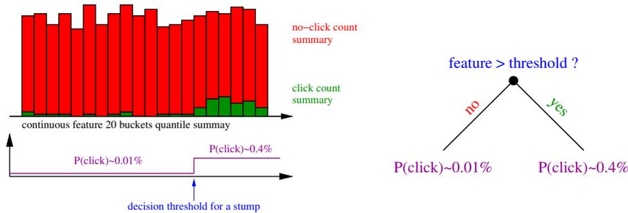
Figure 3: An illustration of how decision stumps are stacked on quantile summaries: the summary maintain a fine grained count of click/no-click for each bucket and the decision stump provides a rougher, but more reliable, CTR estimate.
