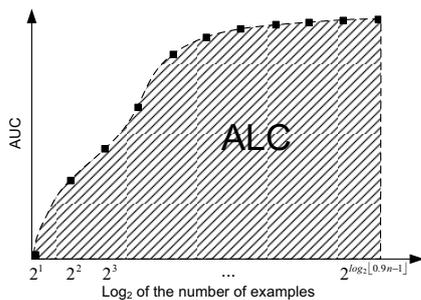
Fig. 3. ALC computation: area under AUC curve
