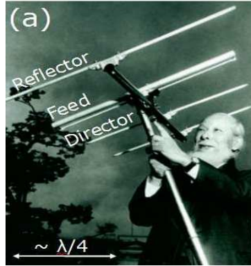
Figure 5.1: A typical Yagi Uda RF antenna held by one of its inventors Hidetsugu Yagi. It has one reflector and two directors(adopted from[141]).
