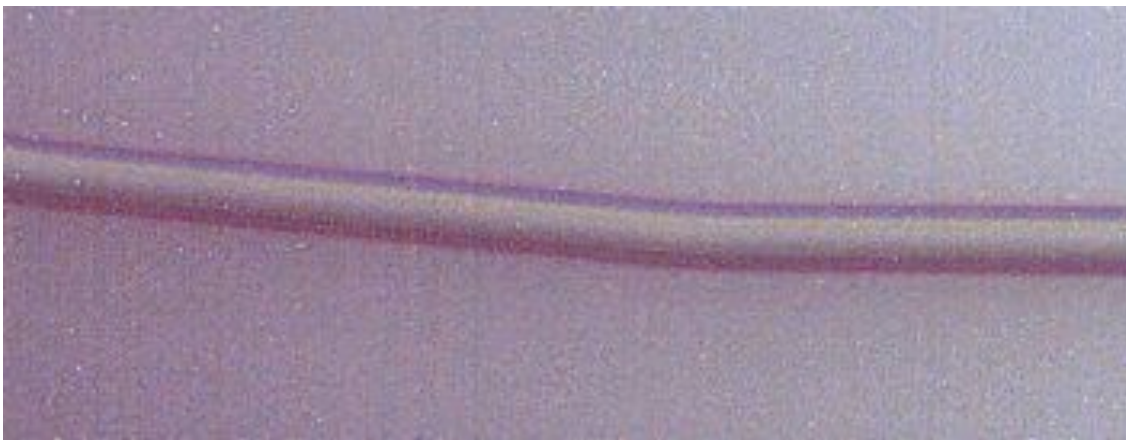
Figure 3.16: "Circularly curved" waveguide with clear discretization of the bend.
