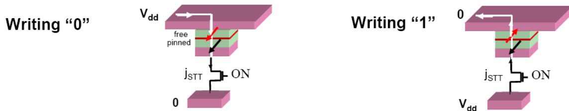
Figure I-9. Schematic of an STT-RAM memory cell.
