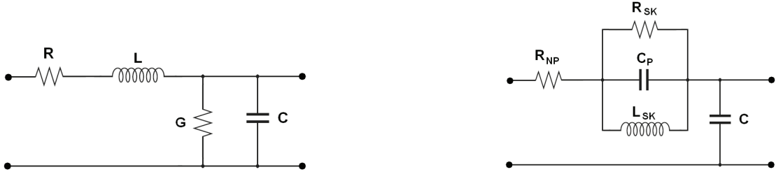
Figure III-30: Equivalent circuit as commonly proposed for transmission lines (left) and our model (right).
