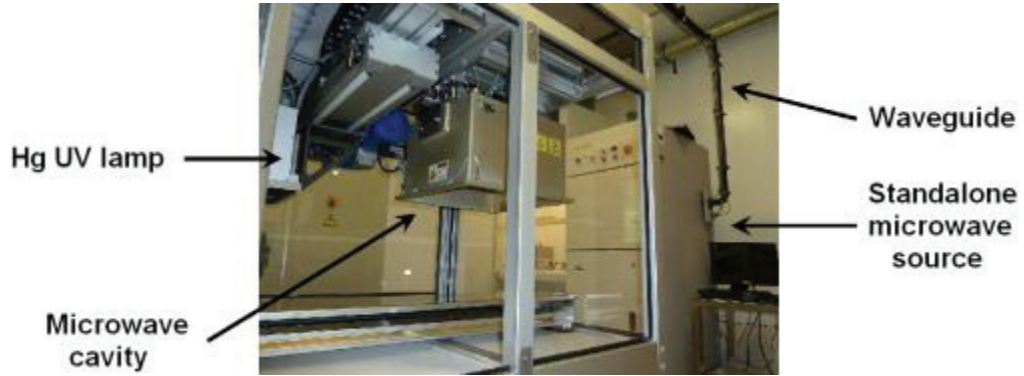
Figure 4: View of the post-treatment equipments integrated in JetPac: UV lamp and microwave cavity in a HVFM configuration.
