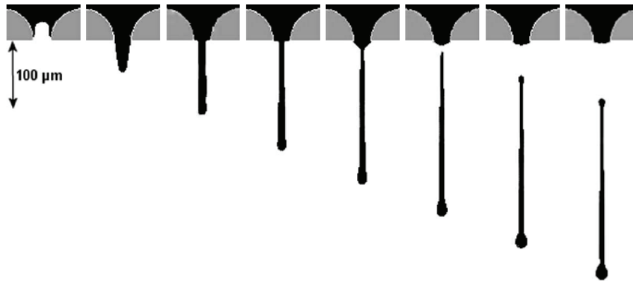
Figure I-23: Sequence of a droplet ejection with a 10 \mu\text{s} timeframe from left to right [96]. In idle state, a slight vacuum depression is applied to maintain the meniscus slightly ingested.
