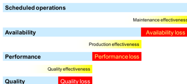
Figure 8 : Illustration of the main components of overall equipment effectiveness (OEE) (Sohal, Olhager, Neill, & Prajogo, 2010)
