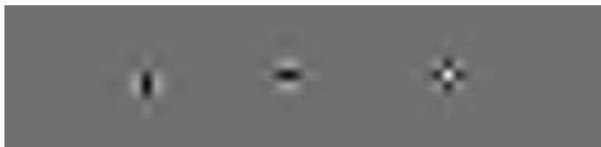
Figure 5.11: Wavelet responses for the first level of a 3-levels CDF 9/7 decomposition. The first two wavelets are oriented in the vertical and horizontal directions. The third wavelet is a mix of two diagonal orientations and gives the “checkerboard” artifact.
