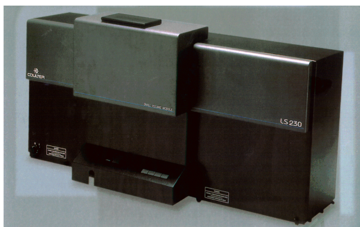
Figure II.1. Photos d'un granulometre laser type coulter LS
