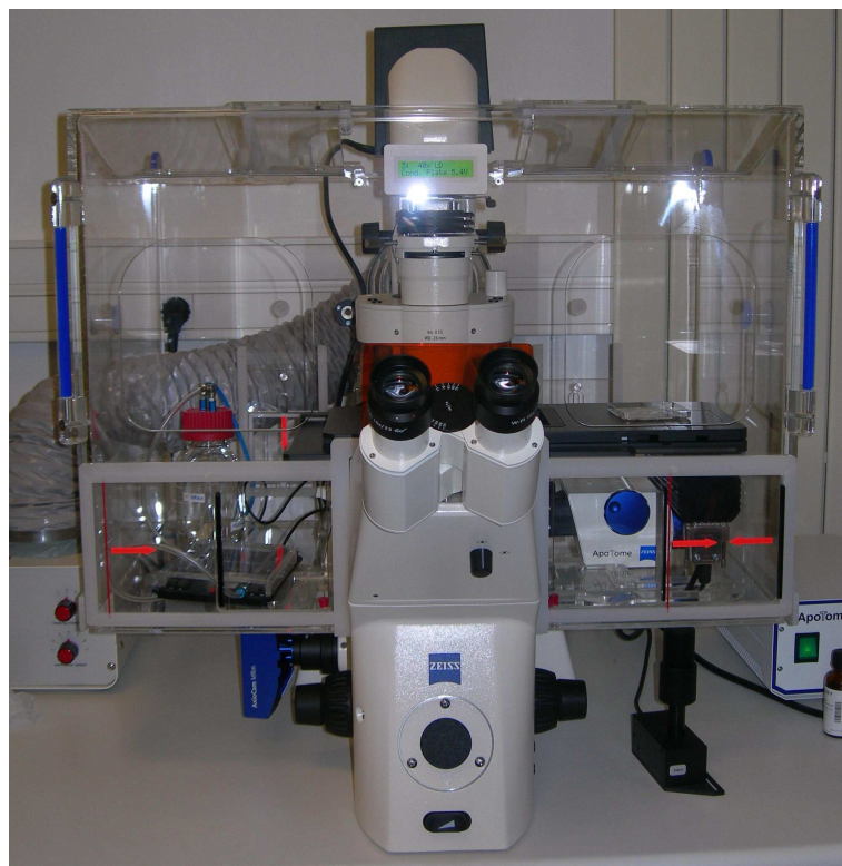
Figure 1.19: Zeiss Axiovert200 microscope with incubation chamber for phase-contrast microscopy, capable of Z-plane photography through the APOTOME system.
