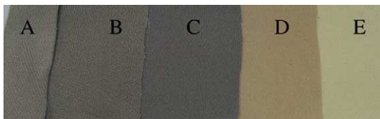
Fig. 3. Samples of plasma-treated textiles with different thicknesses of silver.
