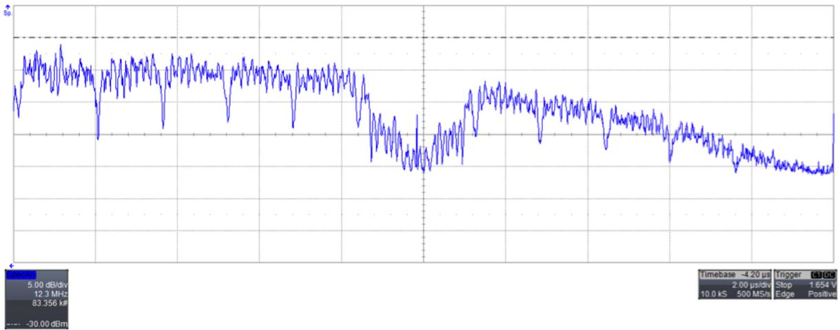
(a) Spectrum of the signal transmitted at the output of the DAC
