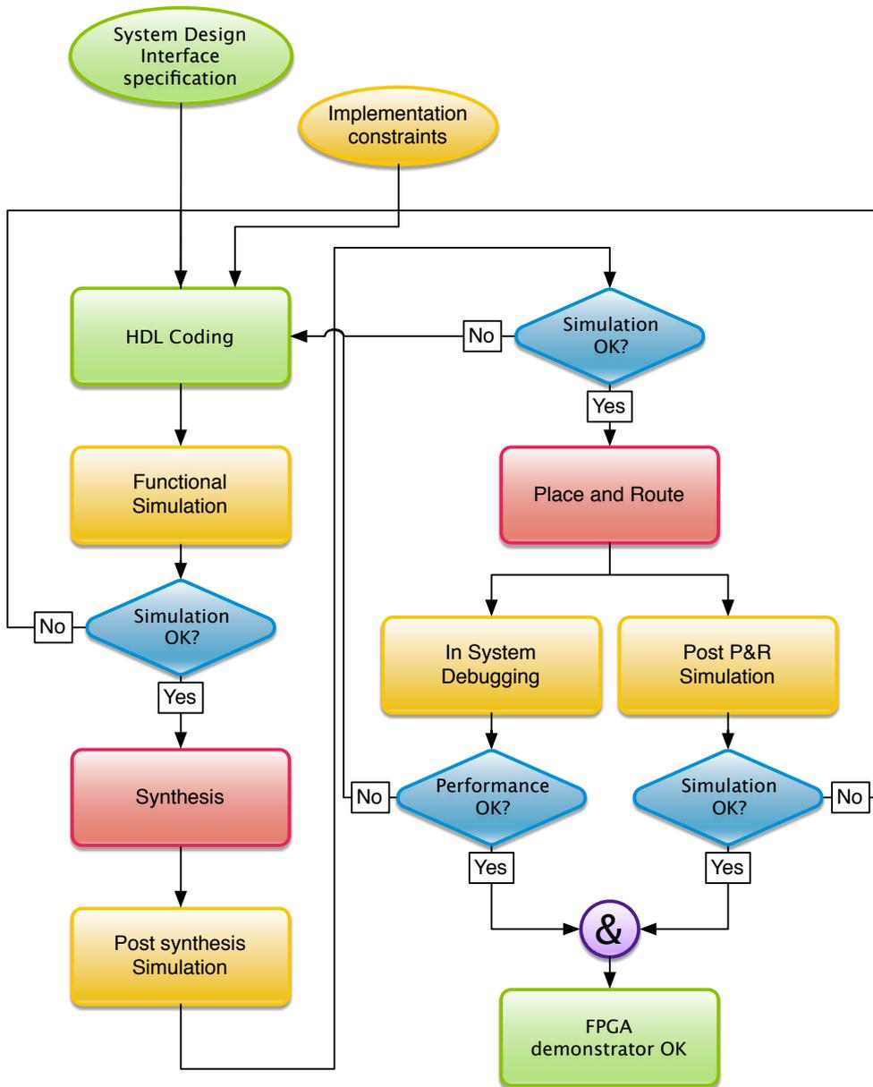
Figure 49: FPGA Flow
