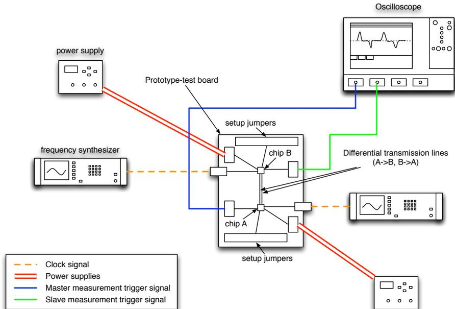
Figure 36: Setup for full connectivity check including PHY TX and RX, MAC, synchronization and localization
