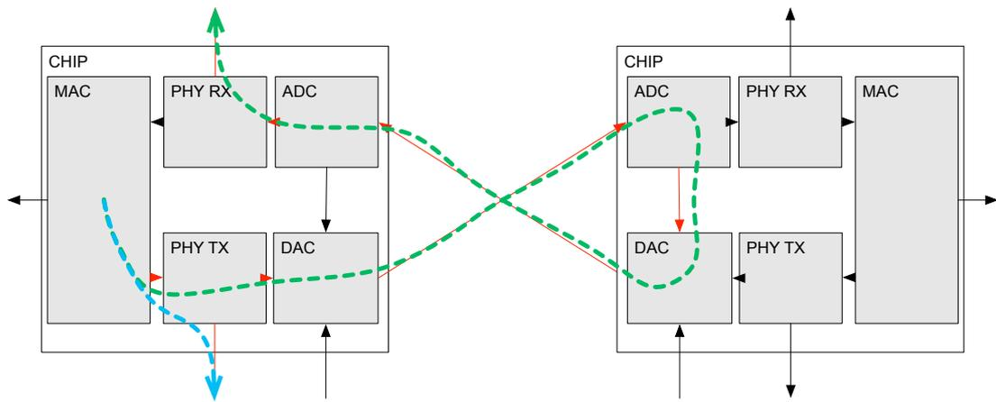
(b) "loopback" test mode for ADC/DAC validation
