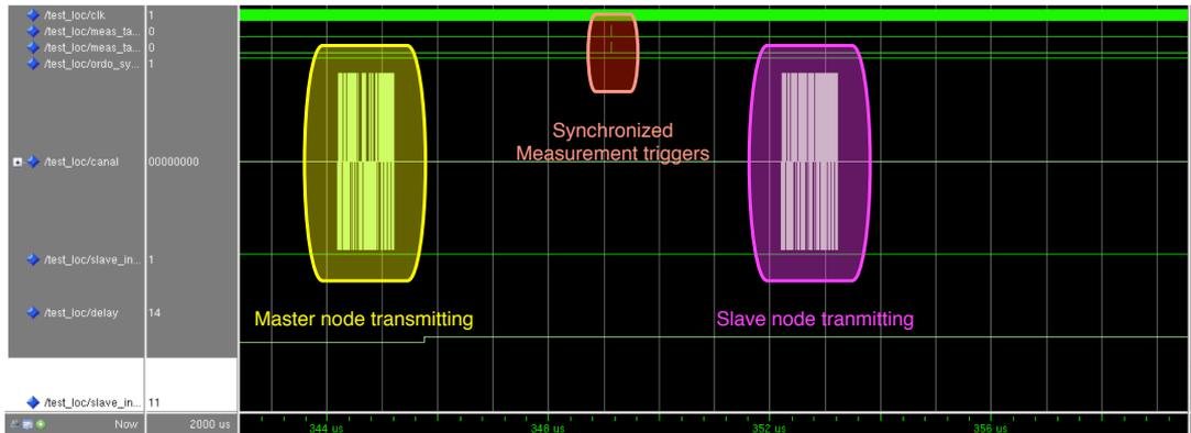
Figure 20: Full working synchronization and localization in hardware simulations
