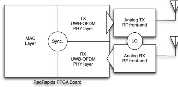
Figure 24: Block diagram of the proposed FPGA demonstrator
