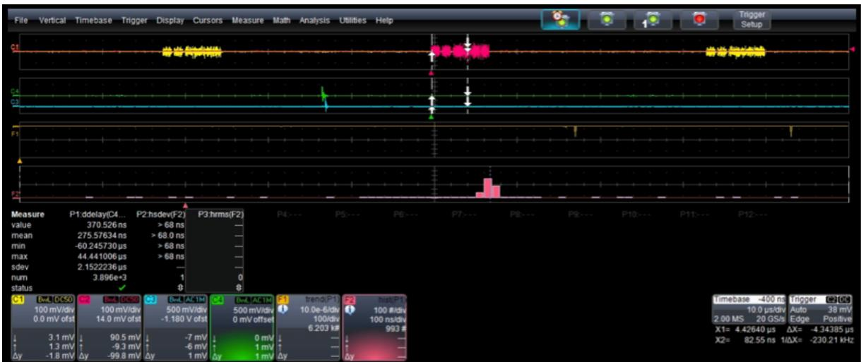
(b) Channel occupation, measurement triggers, and trigger delay statistics
