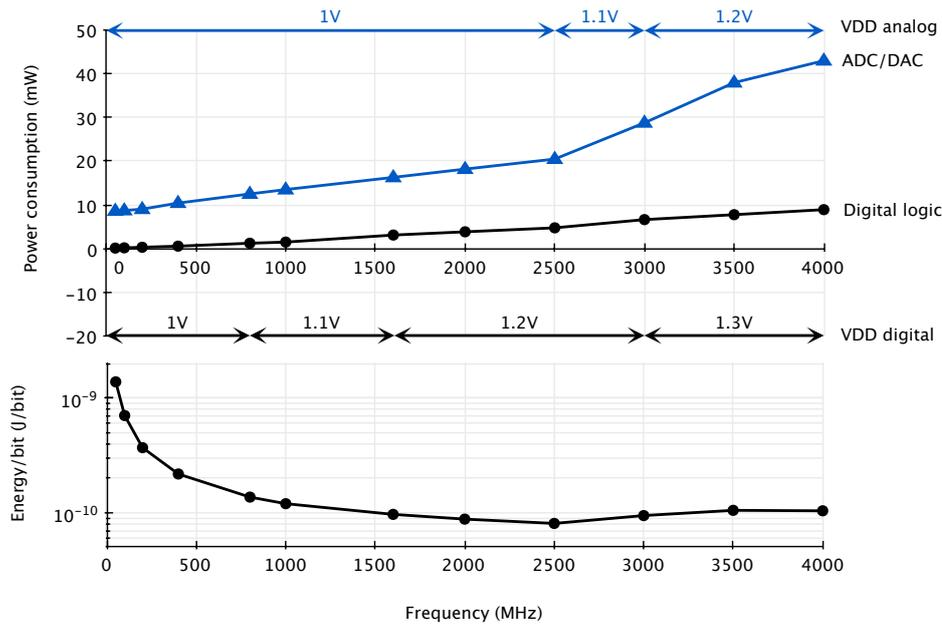
Figure 41: Power consumption versus clock frequency
