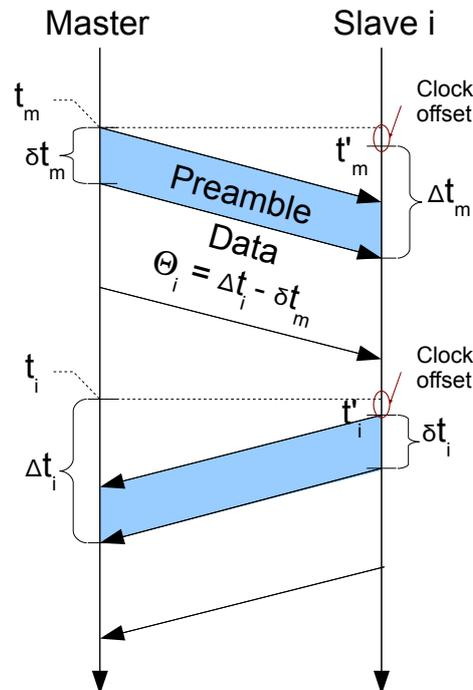
Figure 17: Exchange of timing information
