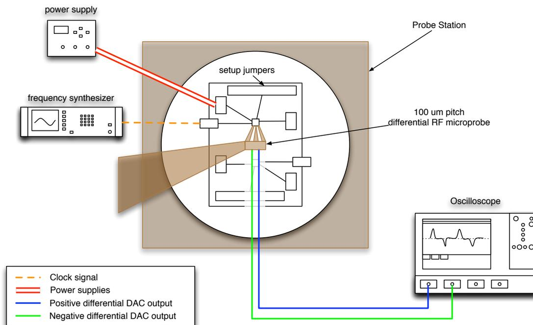
Figure 32: Probe station setup for transmitted signal analysis
