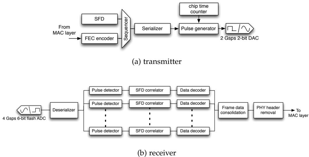
Figure 14: IR-UWB transceiver
