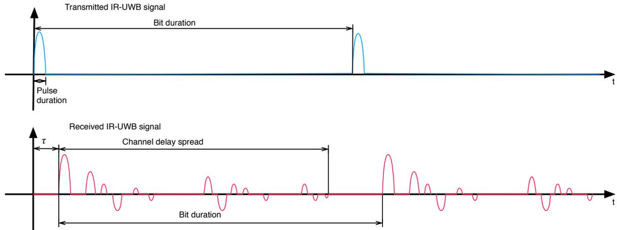
Figure 10: Delay spread of IR-UWB signal
