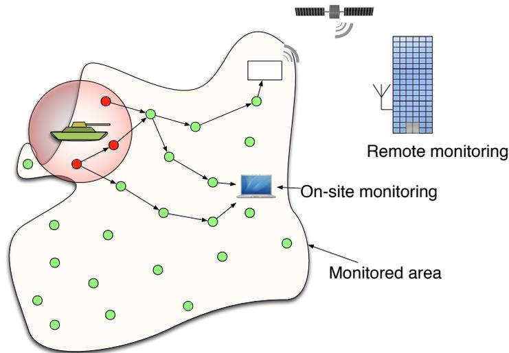
Figure 1: Example of a military oriented intrusion detection system
