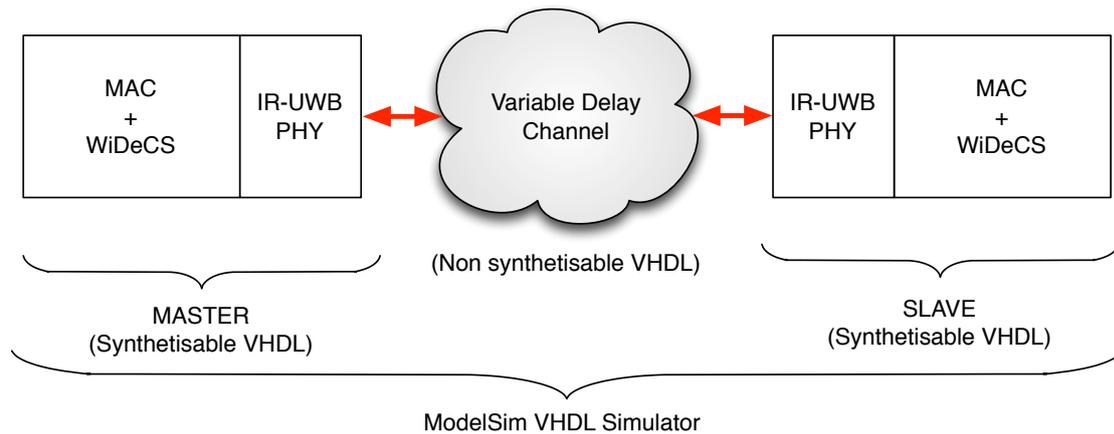
Figure 19: Hardware simulation setup
