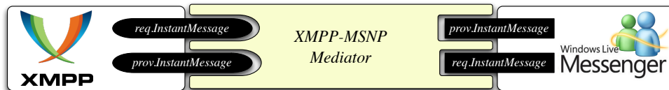
Figure 6.3. Making XMPP and MSNP components interoperable
