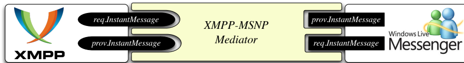
Figure 6.3. Making XMPP and MSNP components interoperable
