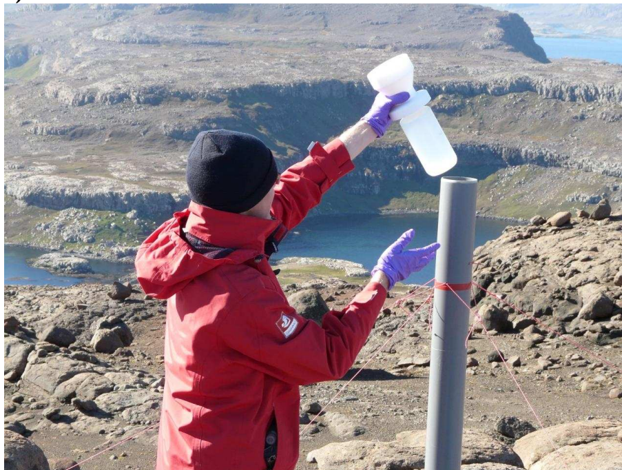
Figure A1-2: (a) Deposition collectors with duplicate sampling and bottle holder pipes; (b) detail of the deposition device.
