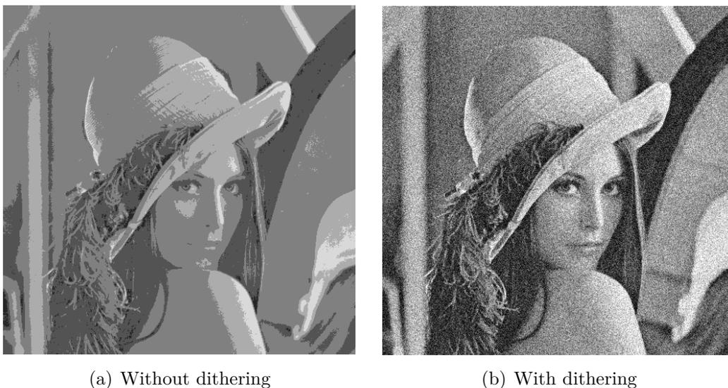
Figure 5.15: Comparison of the reconstruction visual quality between non-dithered and dithered quantizing ganglion cell. The test image is Lena. The observation time is  $t_{obs} = 55ms$ .
