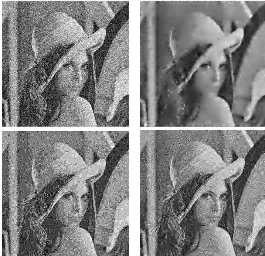
Figure 4.8: Robustness to noise: qualitative comparison between our new codec, JPEG, and JPEG2000 under the same rate restriction (here  $0.27 \text{ bpp}$ ). Upper left: Lena (renormalized in the range of values from 0 to 1) with additive Gaussian noise ( $mean = 0$ ,  $variance = 0.05$ ). Upper right: coded/decoded image using the new codec. Lower left: coded/decoded image using JPEG. Lower right: coded/decoded image using JPEG2000.
