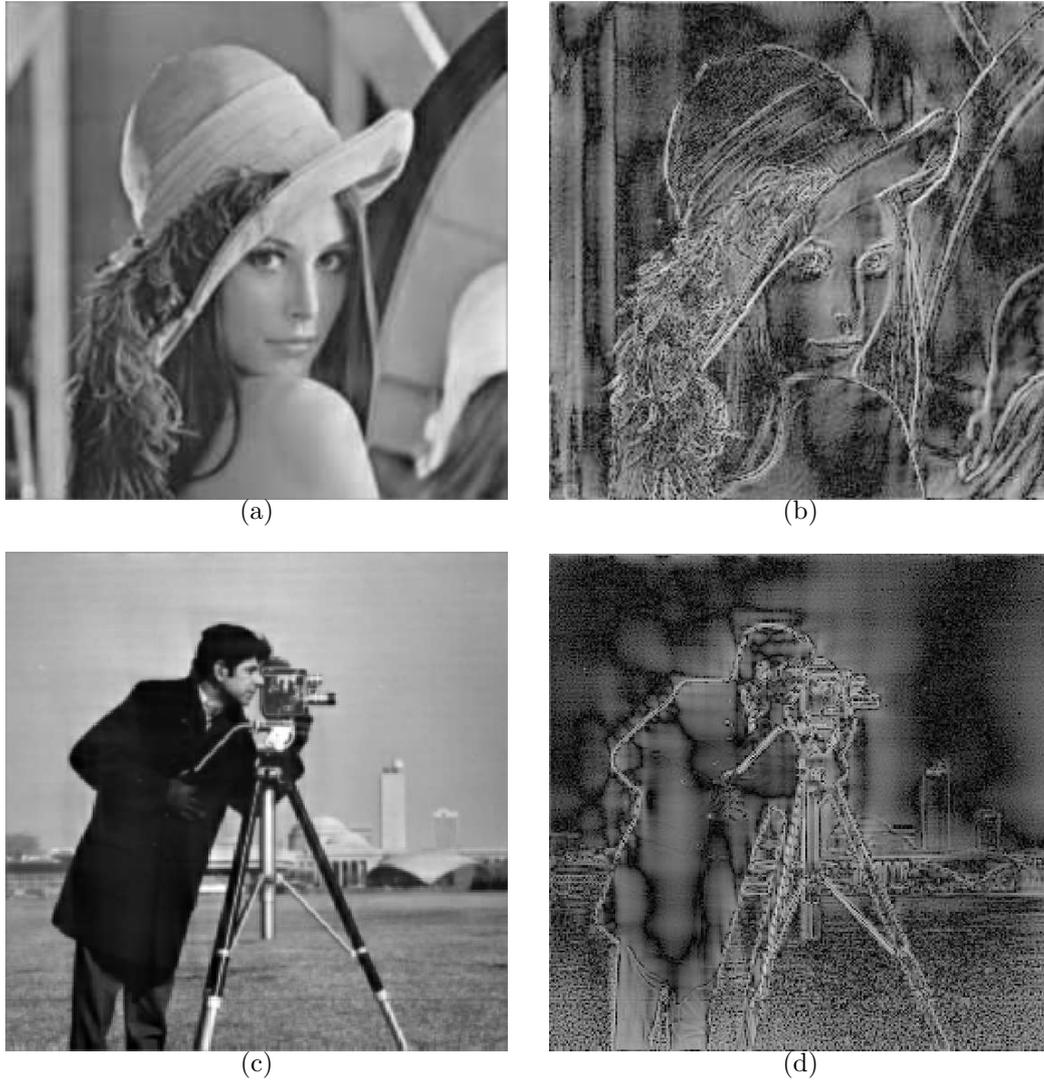
Figure 3.4: Result of the decoding procedure with the equalized moments using the totality of the retina cells. 3.4(a)-3.4(c): Reconstructed images *Lena* and *cameraman*. The PSNR quality measure of  $\tilde{f}_{N_s}^{corr}$  yields 26.8 dB (for *Lena*)/ 27 dB (for *cameraman*). 3.4(d)-3.4(b): Error image shown in a logarithmic scale: high frequencies are the ones that are the most affected by this approach.
