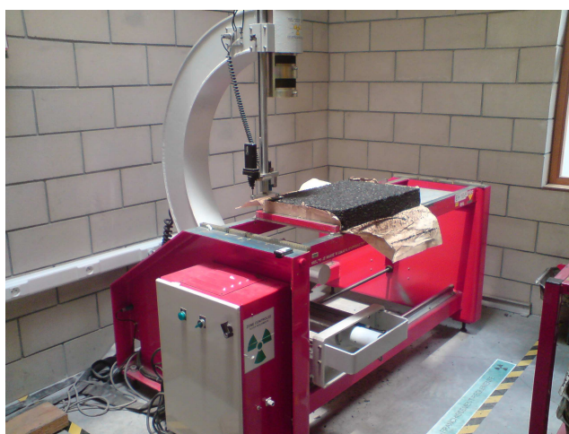
FIGURE B.3 – Banc gamma vertical
