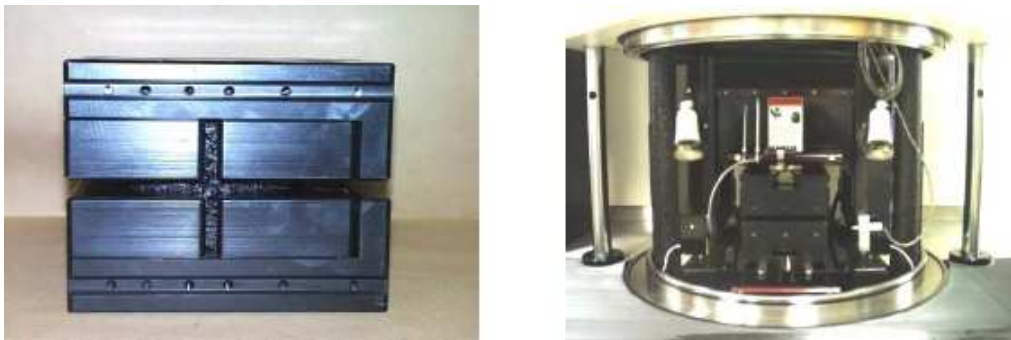
FIGURE 2.6 – Superpave Shear Tester [Mohammad et al., 2002]
