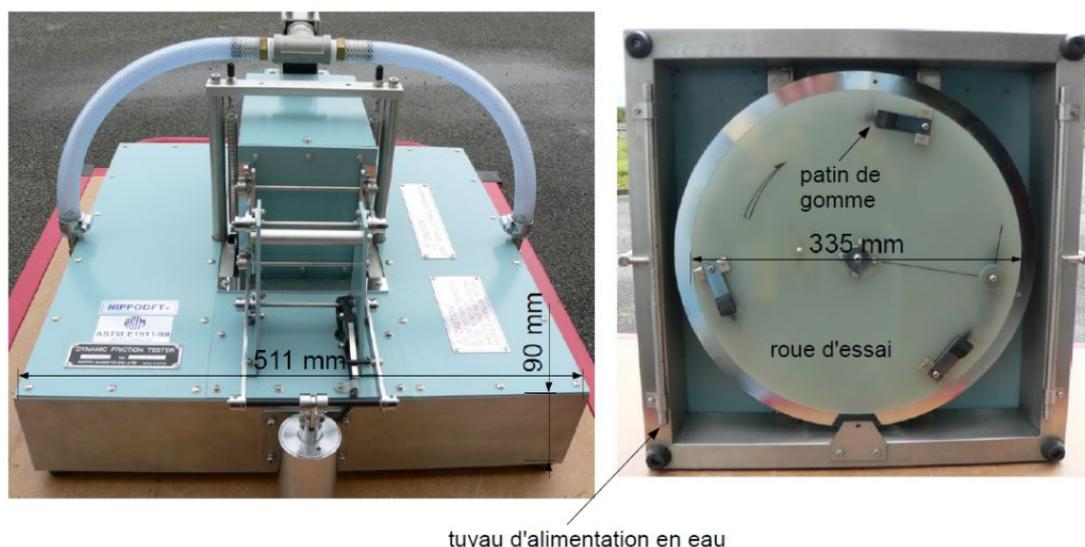
**Figure 1.25** — Le dynamic friction tester *DFT*.
