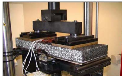
Fig. 2 Five point bending test: above, schematic; below, picture (dimensions are given in Table 1) (adapted from [7])
