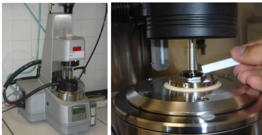
Figure 2. (left) DSR apparatus used for bitumen tests; (right) Close-up on a test sample [EIFFAGE Travaux Publics laboratory, Corbas, France]
