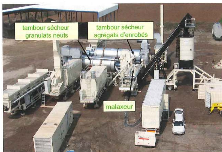
Photo 2 Vue d'ensemble du poste HPR continu General view of HPR continuous mixing plant
