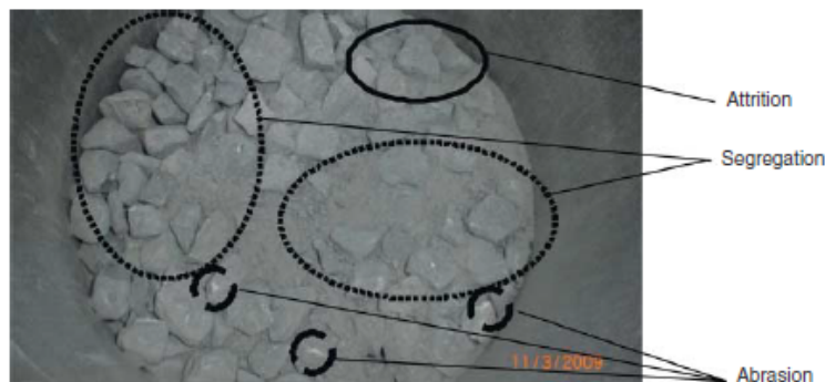
Figure 6. Example of attrition, segregation and abrasion phenomena observed at 100 gyrations using the gyratory shear compactor.
