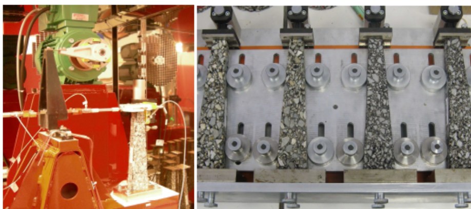
Figure 11. Complex modulus test and fatigue test configuration on trapezoidal specimens (NF EN 12697-24).
