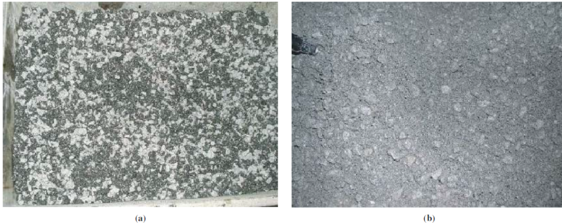
FIGURE 5 Appearance of product for two initial aggregates moistures: (a) mixing at 70°C and 0.84% water and (b) mixing at 70°C and 7% water.
