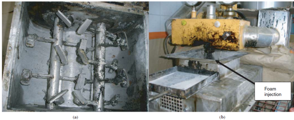
FIGURE 3 Views of (a) SAE mixer and (b) injection of foam into mixer.
