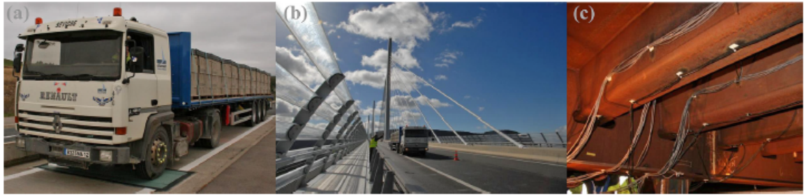
FIG. 5—Pictures of the Millau Viaduct during the experimental measurements: (a) loading truck during weighing, (b) loading truck on the Millau Viaduct, and (c) stiffeners and crossbeam with gauges.
