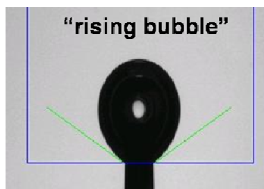
Scheme 3.5 The rising air bubble configuration
