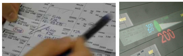
Figure 10: importance of feedback. a) MOD indicates that this strip is a modified and reprinted one; b) feedback for a handwritten heading.
