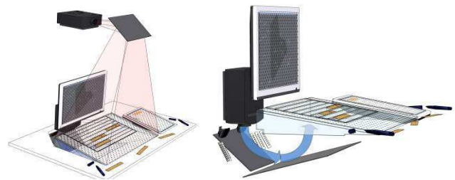
Figure 3: Strip’TIC. Top projector, radar screen, strip board, and side screen (left). Bottom projector casting images on a semi-opaque strip board, two mirrors, infrared LEDs, and webcams (right). Black dots depict pen-sensitive areas.
