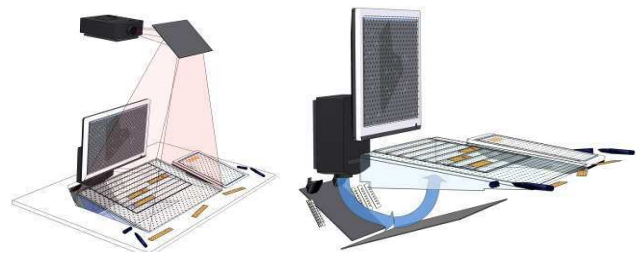
Figure 3: Strip’TIC. Top projector, radar screen, strip board, and side screen (left). Bottom projector casting images on a semi-opaque strip board, two mirrors, infrared LEDs, and webcams (right). Black dots depict pen-sensitive areas.
