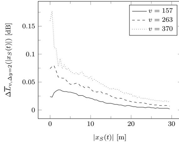
Figure 2.11: Mean values of discrepancies  $\Delta \bar{L}_{v, \Delta y=2}(|x_S(t)|)$  between MTSSM and MTSM for different speeds (in  $\text{kmh}^{-1}$ ). All pass-bys considered.
