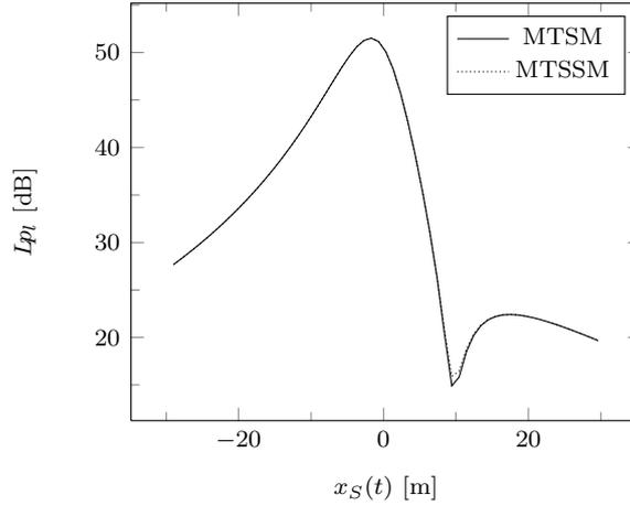
Figure 2.10: Mean-square sound pressure calculated with MTSM and MTSSM. Configuration setup:  $v = 364 \text{ kmh}^{-1}$ ,  $f = 4885 \text{ Hz}$ ,  $\sigma = 5052 \text{ kNsm}^{-4}$ ,  $S(x_S, 5.55, 0.14)$ ,  $M(0, 0, 0.51)$ . A case of large error between MTSM and MTSSM, located at a cancellation.
