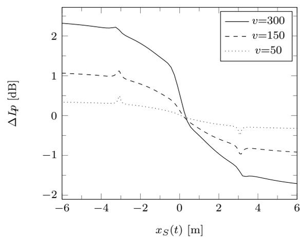
Figure 2.18: Comparison of propagation of the velocity potential and the MTSM pressure signal. Configuration:  $S(x_S, 2, 1)$  is moving above a perfect reflecting ground and is emitting a pure tone at  $f = 1000$  Hz.  $M(0, 0, 1)$ .
