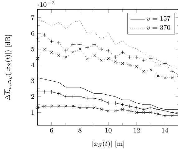
Figure 2.13: Mean discrepancies  $\Delta\bar{L}_{v, \Delta y}(|x_S(t)|)$  between MTSSM and MTSM for different speeds  $v$  in  $\text{kmh}^{-1}$  and  $\Delta y$  (without mark:  $\Delta y = 2$  m, +:  $\Delta y = 4$  m, x:  $\Delta y = 6$  m). All pass-bys considered.
