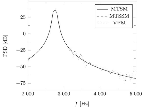
Figure 2.7: Comparison of PSD between the reference model MTSM and two other models MTSSM and VPM. Configuration setup:  $S(4.98, 2, 0.75)$ ,  $M(0, 0, 1)$ ,  $\sigma = 30000$  kNsm $^{-4}$ ,  $v = 130$  kmh $^{-1}$ ,  $f = 3010$  Hz.
