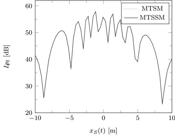
Figure 2.2: Mean-square sound pressure level  $Lp_l$  as a function of  $x_S(t)$  predicted by MTSM and MTSSM. Configuration setup:  $S(x_S, 2, 0.75)$ ,  $M(0, 0, 1)$ ,  $\sigma = 30000 \text{ kNsm}^{-4}$ ,  $v = 130 \text{ kmh}^{-1}$ ,  $f = 3010 \text{ Hz}$ .
