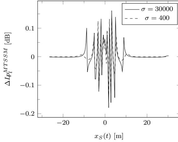
Figure 2.4: Mean-square sound pressure differences between MTSSM and MTSM as a function of  $x_S$ . Configuration setup:  $S(x_S, 2, 0.75)$ ,  $M(0, 0, 1)$ ,  $\sigma = 30000 \text{ kNsm}^{-4}$ ,  $v = 130 \text{ kmh}^{-1}$ ,  $f = 3010 \text{ Hz}$ .
