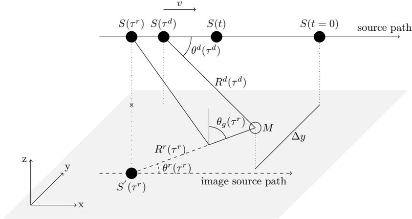
Figure 2.1: Moving sound source  $S$  with its image source  $S'$  and a motionless receiver  $M$ .
