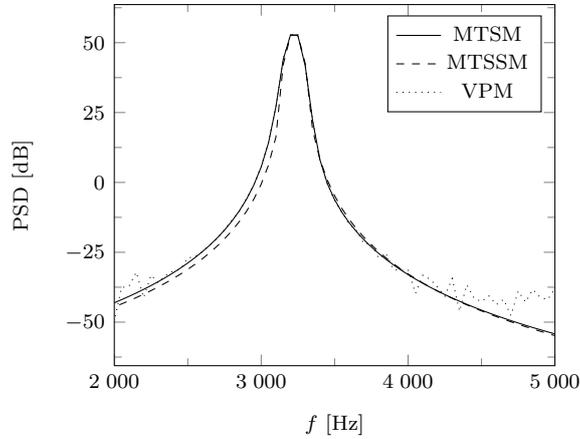
Figure 2.6: Comparison of PSD between the reference model MTSM and other two models MTSSM and VPM. Configuration setup:  $S(-1.52, 2, 0.75)$ ,  $M(0, 0, 1)$ ,  $\sigma = 30000$  kNsm $^{-4}$ ,  $v = 130$  kmh $^{-1}$ ,  $f = 3010$  Hz.  $x_S$  is chosen so that  $|\sqrt{\tilde{c}^d} - \sqrt{\tilde{c}^r}|$  is maximum, for higher discrepancies.
