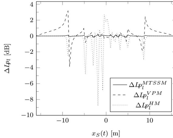
Figure 2.5: Mean-square sound pressure differences between MTSSM or VPM or HM and MTSM as a function of  $S$ -abscissa. Configuration setup:  $S(x_S, 2, 0.75)$ ,  $M(0, 0, 1)$ ,  $\sigma = 30000 \text{ kNsm}^{-4}$ ,  $v = 130 \text{ kmh}^{-1}$ ,  $f = 3010 \text{ Hz}$ .
