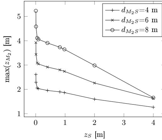
FIGURE 4.6 – Maximum height of  $M_2$  that ensures the empirical criterion  $\delta \geq 0.001$  m, as a function of the source height and for 3 distances from the source.  $M_1(z_{M_1}=1 \text{ m}, d_1=2 \text{ m})$ .
