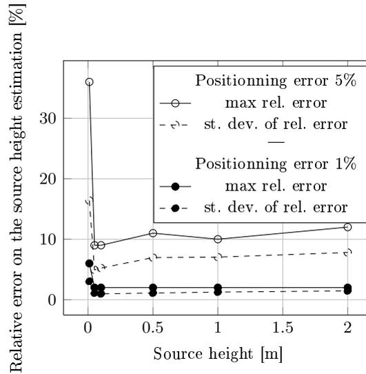
FIGURE 4.7 – Maximum and standard deviation of the relative error on the source height estimation, for a precise and less precise positioning (resp. 1% and 5% error on positioning) of microphones. Standard positioning :  $(z_{M_1}, d_1, z_{M_2}, d_2) = (1 \text{ m}, 2 \text{ m}, 1 \text{ m}, 4 \text{ m})$ .
