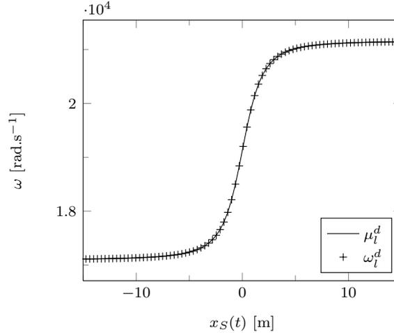
Figure 2.8: Comparison of  $\mu_l^d$  and  $\omega_l^d$ . Configuration setup:  $S(x_S, 2, 0.75)$ ,  $M(0, 0, 1)$ ,  $\sigma = 30000 \text{ kNsm}^{-4}$ ,  $v = 130 \text{ kmh}^{-1}$ ,  $f = 3010 \text{ Hz}$ .
