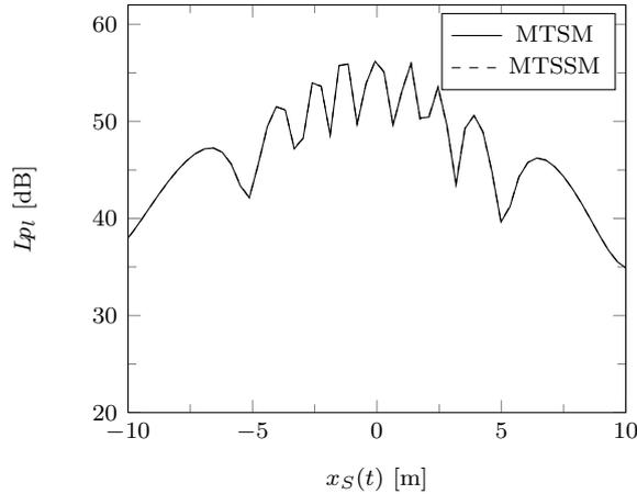
Figure 2.3: Mean-square sound pressure as a function of  $x_S(t)$  predicted by MTSM and MTSSM. Configuration setup:  $S(x_S, 2, 0.75)$ ,  $M(0, 0, 1)$ ,  $\sigma = 400 \text{ kNsm}^{-4}$ ,  $v = 130 \text{ kmh}^{-1}$ ,  $f = 3010 \text{ Hz}$ .
