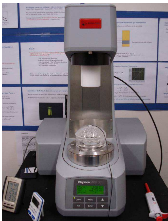
Fig. 2.9: View of the Anton Paar MCR301 rheometer in the absence of the upper rotor but with the plexiglass hood chamber during a temperature calibration test (wire is the one of an external temperature controller).
