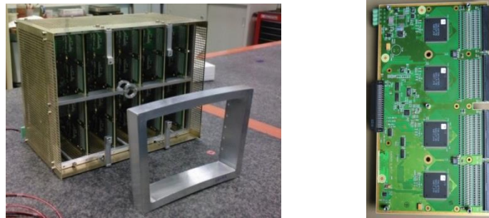
Figure 3-17. The T2K electronics. (a) the packaging of electronics for one module test; (b) one FEC ( 14\text{ cm} \times 25\text{ cm} ).
