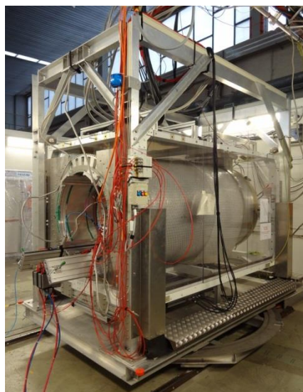
Figure 3-1. Large Prototype (LP) with the movable stage in the beam area.
