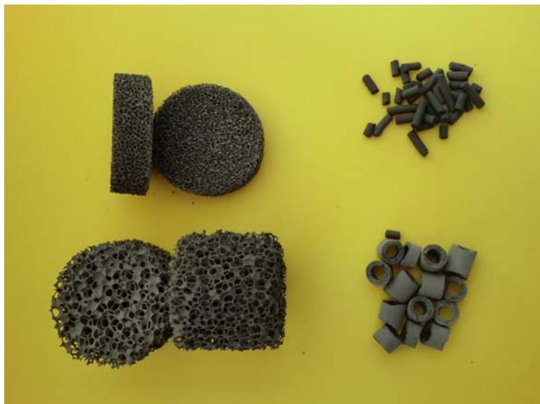
**Figure 9.** Silicon carbide (SiC) with different shapes synthesized by the gas-solid reaction (courtesy by Sicat).
