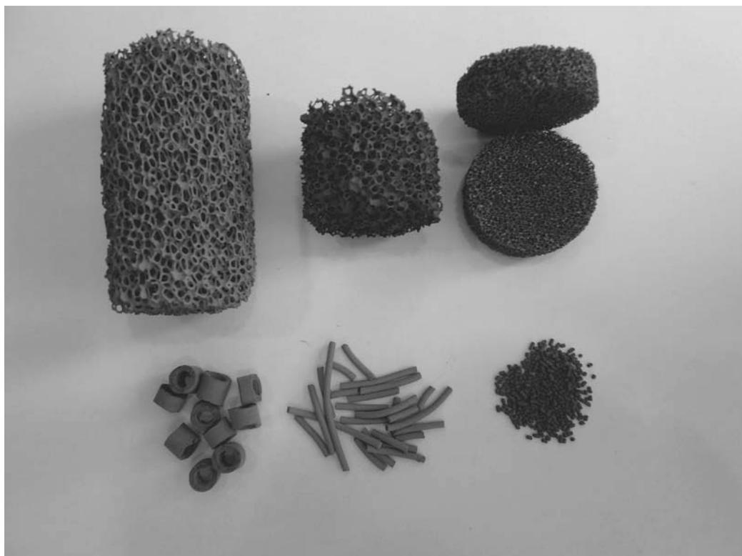
**Figure 1.** Silicon carbide ( $\beta$ -SiC) with different size and shape synthesized via a gas-solid reaction (courtesy by [www.sicatcatalyst.com](http://www.sicatcatalyst.com)).
