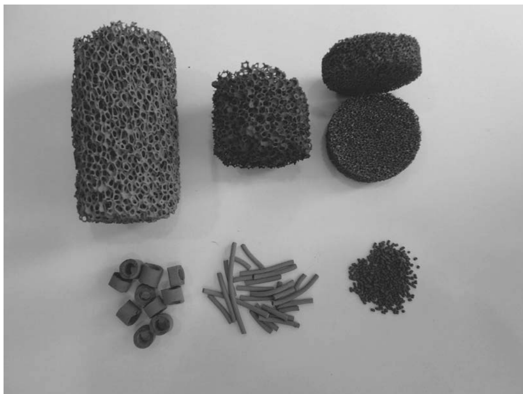
Figure 1. Silicon carbide ( \beta -SiC) with different size and shape synthesized via a gas-solid reaction (courtesy by www.sicatcatalyst.com ).
