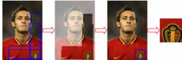
Figure 8.3: Steps to obtain the suggested visual object on an image from BelgaLogos: i) selecting the bounding box, ii) intersection of bounding box , iii) keeping only the region that have been covered by at least two bounding box. The final result is the suggested object.
