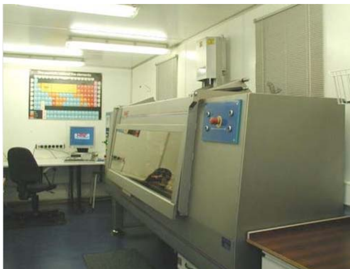
Figure Y: Scanner Avaatech XRF du Royal Netherland Institute for sea Research (image laboratoire NIOZ)
