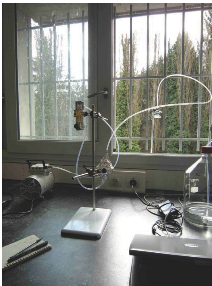
FIGURE 2.2 - Photograph of the sampling apparatus in operation in Grenoble, France. The active ozone sampler consists of 1/4" PFA tubing connecting three main sampler components: (i) a standard low-volume vacuum pump ( bottom left ) equipped with a needle valve/flow meter ( top center ); (ii) a closed PFA filter holder assembly containing a nitrite-coated filter, covered in aluminum foil ( bottom center ); and (iii) an open-faced filter holder assembly containing a PTFE prefilter for the removal of particulate matter ( top right ).
