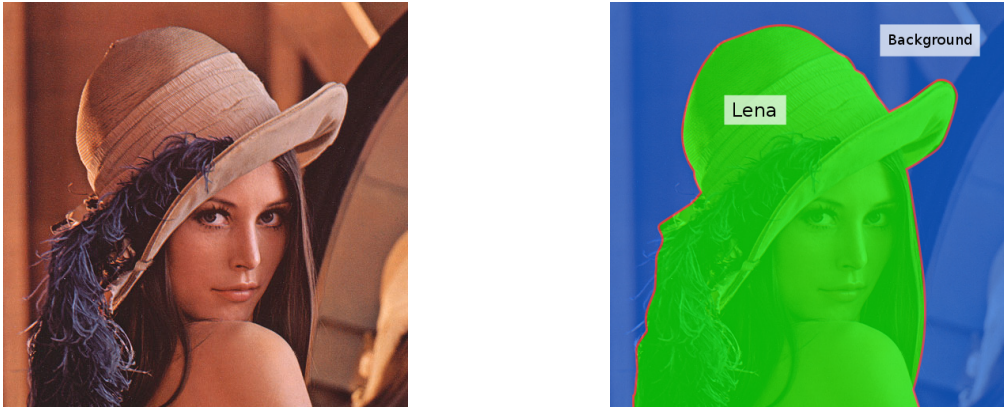
Figure 1.1.3 – Image segmentation example. (left) Original image; (right) Segmented image. This segmentation is visualized by a boundary (red curve) separating the two regions and different colors assigned to the pixels, one per segment.
