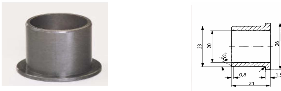
Figure 2.31. Palier lisse GFM - 202326 - 21
