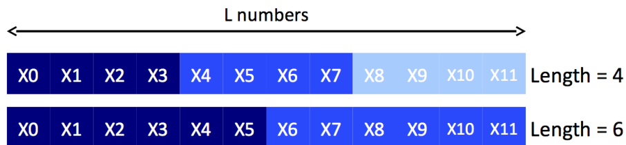
Figure 2.1: Sequence splitting in a unique original stream considering 2 processing elements (PEs), then 3 PEs
