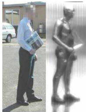
Fig. 1.8: Passive imaging at 94 GHz from QinetiQ [13]
