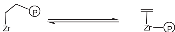
Scheme I.7: Ziegler-Natta polymerisation and depolymerisation mechanism over [\text{Zr-H}] , with \text{Zr-H} = [(\equiv\text{SiO})_{(4-x)}\text{ZrH}_x]/ x= 1 or 2 . [9]
