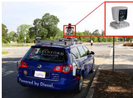
Figure 4.25. "Junior", the autonomous car used for data collection. The Velodyne laser rangefinder mounted on the roof top provides a 3D point cloud of the car surroundings.
