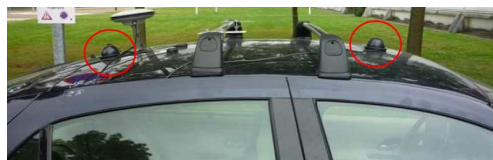
Figure 4.13. Antenna placement on the test vehicles.
