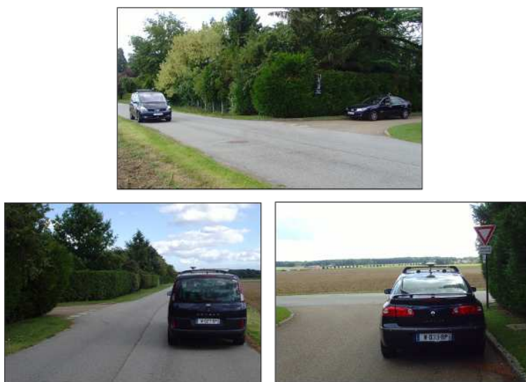
Figure 4.11. Test intersection in Guyancourt: T-shaped give-way intersection. The view is obstructed by the vegetation, therefore the drivers cannot see each other while approaching the intersection.
