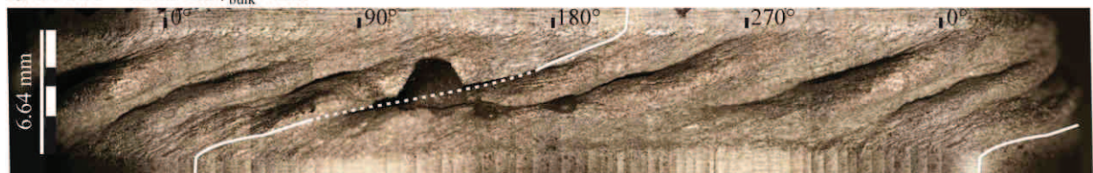
Figure V* 8 : Reconstructed panorama displaying the external appearance of twisted samples still embedded in their iron jacket. The black and white rectangles represent the mafic and felsic initial distribution. The number in mm is the sample length, measured after experiments. Strain markers have been highlighted by a white line (dashed when not visible) and reveal the strain distribution across the sample. For the PP156 experiment conducted at 1160°C, the strain is heterogeneously distributed and was locally calculated (triangles). Other experiments show a homogeneous strain distribution.
