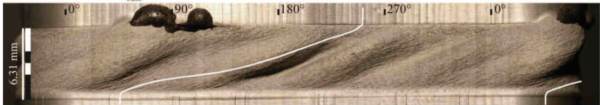
d) PP161 - 1170°C, \gamma_{\text{bulk}} = 3.1
