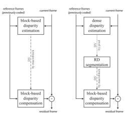
Figure 1.4: Disparity prediction: (left) block-based estimation, (right) enhanced by a dense estimation.
