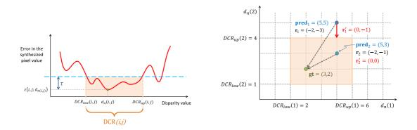
Figure 1.6: Left: Definition of DCR for a given threshold  $\tau$ . Right: Coding the residuals using DCR with a toy example with just two pixels ( $d_n(1)$  and  $d_n(2)$ ). In conventional coding, given predictor (**pred**), one aims to reconstruct the original ground truth (**gt**). However, considering DCR, it is sufficient to encode a generally smaller residual, i.e. one that enables to reconstruct a value inside or on the border of the DCR (shaded area in the picture).
