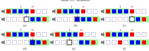
Figure 3.8: Strategies for IMVS with N = 4 and m = k + 2: (a) A-DIBR; (b) A-DIBR; (c) I-DIBR; (d) I-DIBRc; (e) GOPp; (f) noDIBR. The KFs are in red and the WZFs in blue. The frames with green background are displayed. The filled frames are sent by the video server to the user. The black arrow shows that DIBR is applied.
