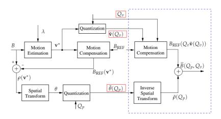
Figure 1.1: The new coding mode operation. In red: the information sent to the decoder, represented by the dashed box. The reference information  $B_{\text{REF}}$  is known both by the encoder and the decoder.
