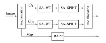
Figure 2.1: Object-based coding scheme
