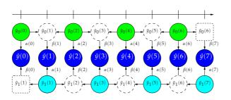
Figure 3.6: Structure of central decoder. Solid circles represent received frames; dashed circles represent interpolated frames. Horizontal arrows represent interpolation. Vertical arrows represent weighted sum. With  $\hat{y}_n(k)$  we denote the *k*-th frame of description *n*. For each *k*,  $\beta(k) = 1 - \alpha(k)$ .
