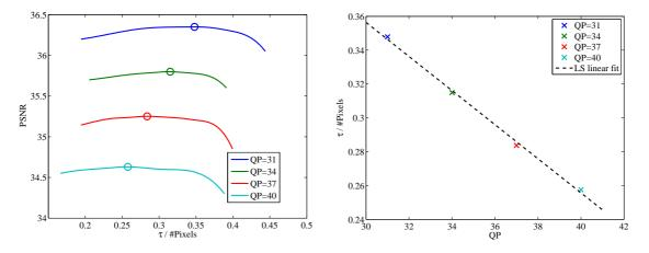
Figure 1.5: Left: Effect of  $\tau$  (normalized over the number of image pixels) on the disparity quality, for several values of the quantization step. Right: Best normalized  $\tau$  values in function of QP. The best fitting first order polynomial is shown as well.
