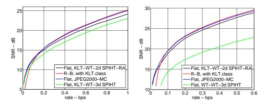
Figure 2.3: Rate-distortion performance of shape adaptive coding algorithms
