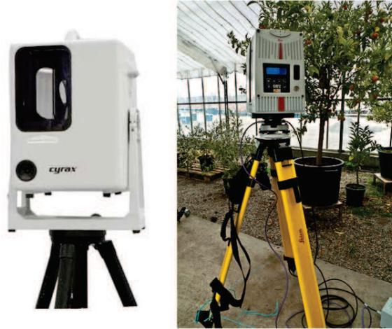
Figure 4.1: The laser scanners: Leica Geosystems HDS2500 (left) , and Leica Geosystems HDS6200 (right).
