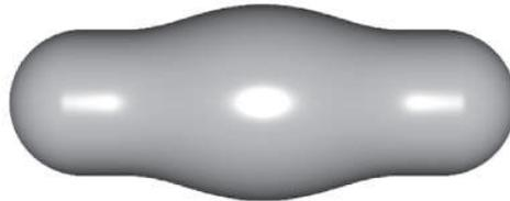
Figure 2.19: Bulge when two line segments with coincident end points are blended. [Galbraith *et al.* 2004]
