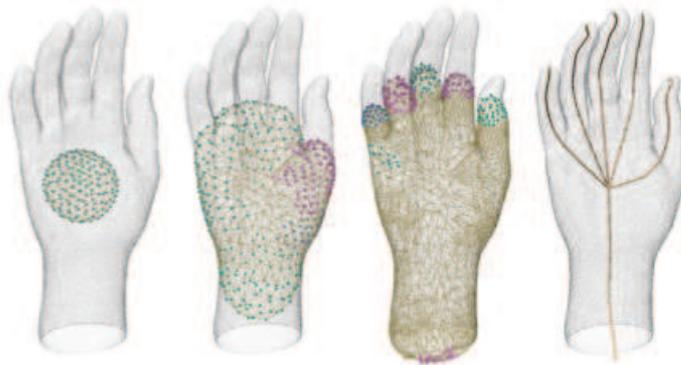
Figure 1.29: Computation of cross-section plane for each sample point. Starting from an initial cutting plane (left), the algorithm iteratively re-estimate the plane (right) using a local optimization. [Sharf *et al.* 2007]
