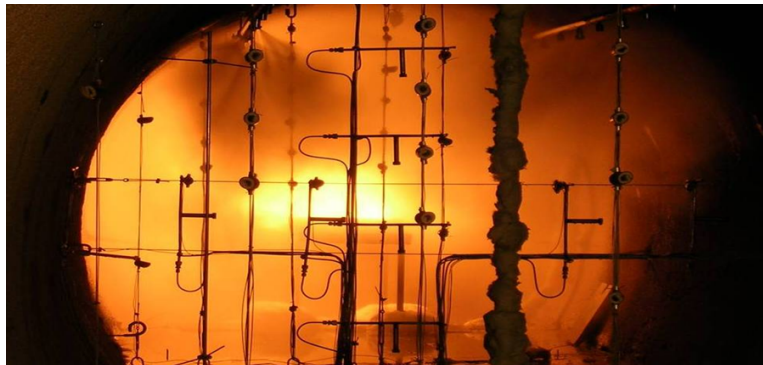
Water spray during a fire test conducted in the midscale tunnel at CSTB
