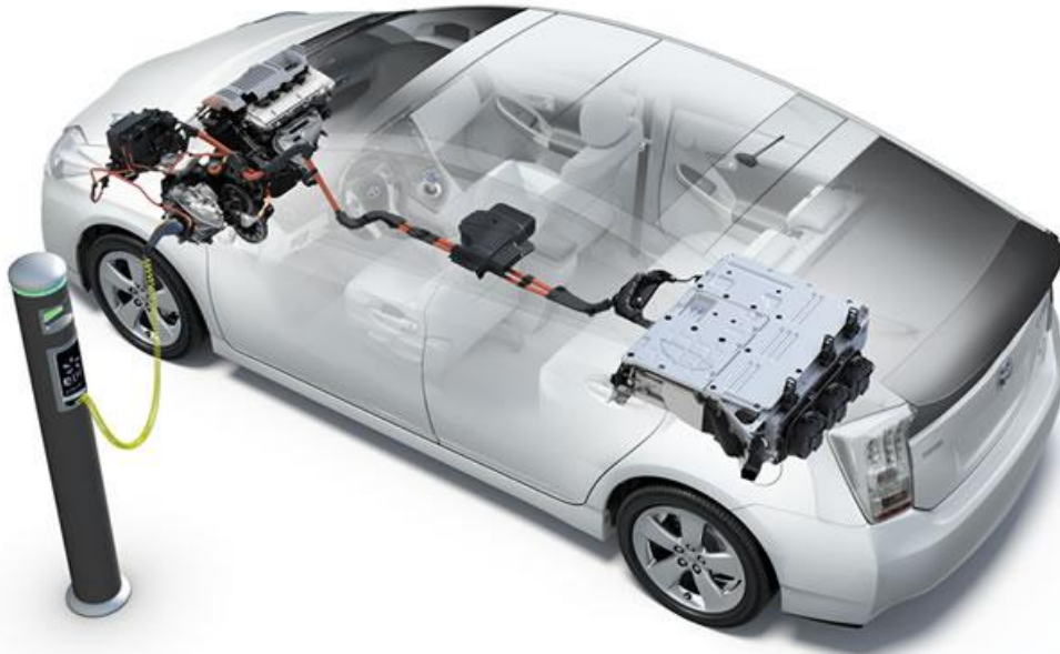
Figure 1.15 : Architecture Toyota Prius rechargeable.
