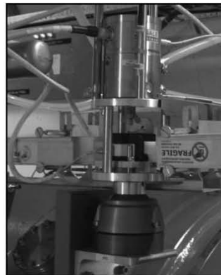
2 Hydrostatic levelling system sensor in LHC environment. Dimensions are: 140 mm height, 100 mm of diameter
